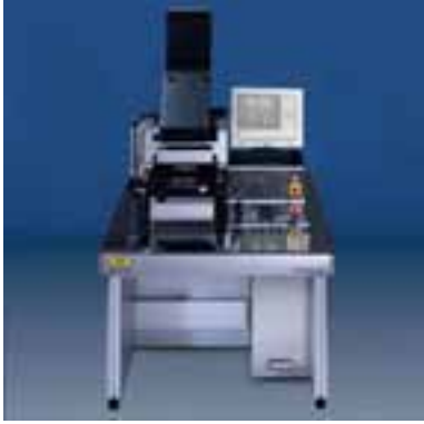
Fig. 1: Semi-automated EVG620 soft UV-NIL system for R&D and pilot line production
