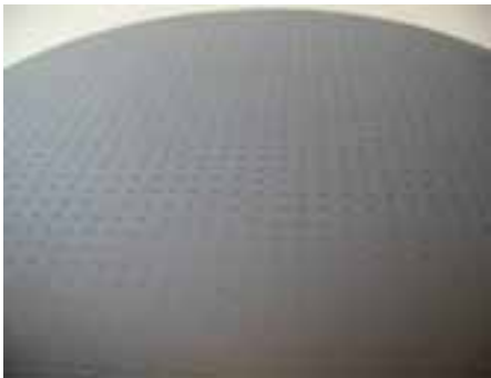
Figure 8: Image of an array of micro-lenses (diameter of lenses: 1 mm, height of lenses: 500 \mu\text{m} ) imprinted with working stamp on 200 mm glass wafers
